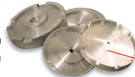
Aluminum bonder dies heat faster and more evenly than steel.
